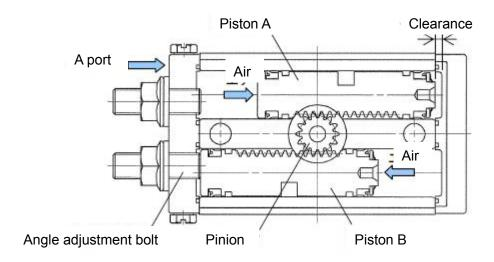
As explained above, this phenomenon occurs when the product uses the angle adjustment bolt. In other words, the halving of the torque can be avoided by adjusting the angle using external stoppers that prevent the piston coming into contact with the adjustment bolt.
